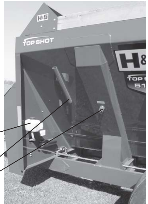
The oiler reservoir is located on the left front side by the scraper holder and jack storage position.
