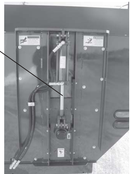
The discharge gate control cylinder shaft and both front and rear main auger cylinders should also be frequently coated with a rust preventative spray or lubricate since the cylinder shaft may remain extended when not being used for a period of time.
