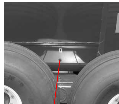
Single or Tandem Axle Wheel Pivot (Each Side)
