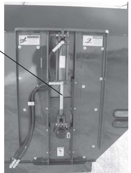
The discharge gate control cylinder shaft and both front and rear main auger cylinders should also be frequently coated with a rust preventative spray or lubricant since the cylinder shaft may remain extended when not being used for a period of time.
