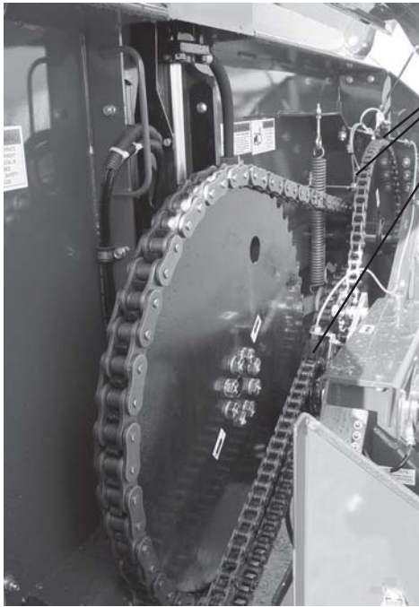
The oiler reservoir is located on the left front side by the scraper holder and jack storage position.
