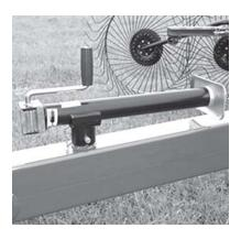
3. Connect the 2 hydraulic hoses for raising and lowering rake arms to the tractor. Open the 2 hydraulic transport lock valves and operate the tractor valve to fill the hydraulic lines and operate the cylinders. Add hydraulic fluid to the tractor system, as required.
