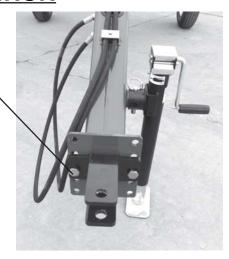
2. Remove the weight from the lift jack. Place the jack in the storage position.
