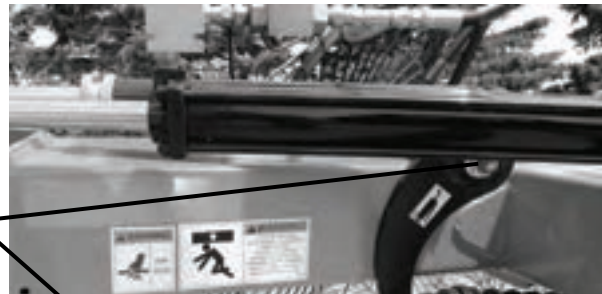
1 zerk on each of the pivot points
