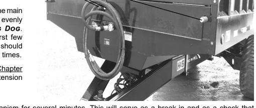
Run the unloading mechanism for several minutes. This will serve as a break-in and as a check that all parts are assembled and lubricated properly. Successful operation will be achieved by periodic adjustments and experience of the operator.
