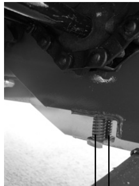
Rear Center Main Apron Tightener Bolts
