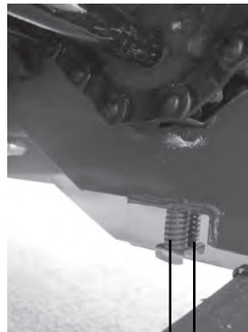
Rear Center Main Apron Tightener Bolts
