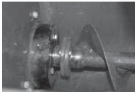
Transfer Auger Front Bearing (under mill cover, 1 zerk on front bearing)
