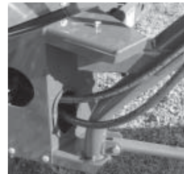
SIA Upper Pivot Bearing (1 zerk) SIA Lower Pivot Bearing (1 zerk)
