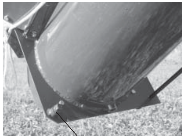
SIA Drain Plug In Storage Position.
