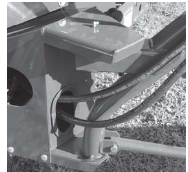
SIA Upper Pivot Bearing (1 zerk)
