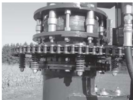
Unloading Auger Pivot/Collar (4 zerks - 2 on the top of the collar & 2 on the bottom of the collar)
