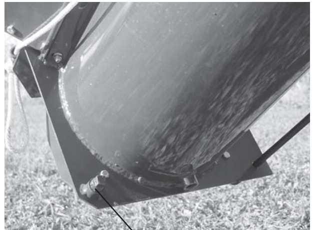
SIA Drain Plug In Storage Position.
