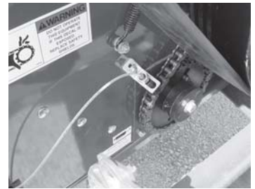
Auger/Transmission Main Shear Bolt(1 zerk)
