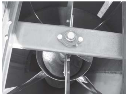
Top of Mixing Auger (1 zerk - under top of tank cover)
