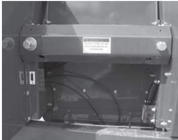
*Front & Rear Mill Bearings (2 zerks)
