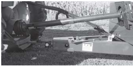
Telescoping PTO Drive (3 zerks)
