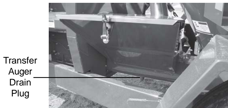
Transfer Auger Drain Plug In Storage Position.
