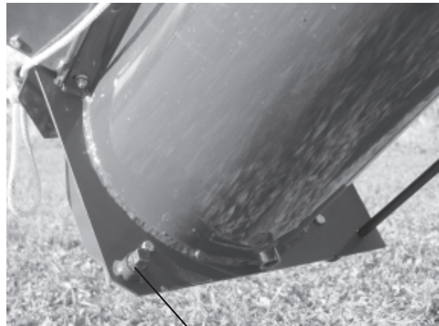
SIA Drain Plug In Storage Position.
