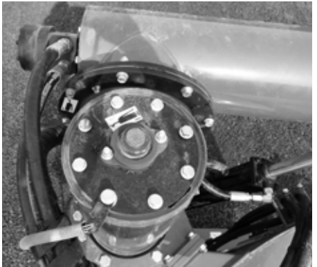
Unloading Auger (1 zerk on the top of vertical section auger and 4 zerks on vertical auger pivot.)
