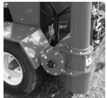
#1 Discharge Auger End Bearing (1 zerk)
