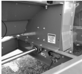
Main Drive Shaft Intermediate Bearing (1 zerk under shield)
