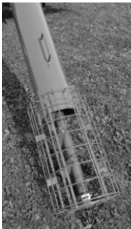
Intake Auger (1 zerk)
