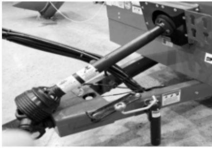
Telescoping PTO Drive (3 zerks) Jack (1 zerk)
