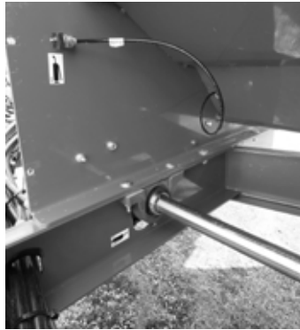
Transfer Auger & Main Drive Shaft Front Bearings (1 zerk each under shield)
