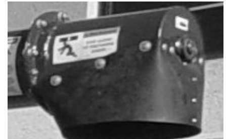
Unloading Auger - (1 zerk at the end of the auger discharge spout)
