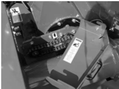
#1 Discharge Auger Bearing (1 zerk under shield)
