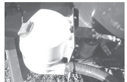
Oil level should be between Max/Min level marks
