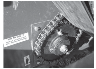
Auger/Transmission Main Shear Bolt-(1 zerk)
