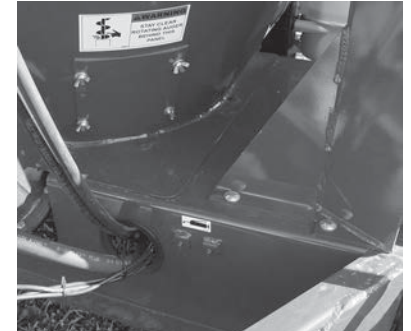
Transfer Auger Rear Bearing (1 zerk - remote on rear of frame)
