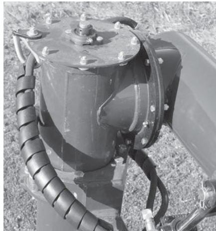
Unloading Auger-(1 zerk on the top of vertical section auger and 4 zerks on vertical auger pivot.)
