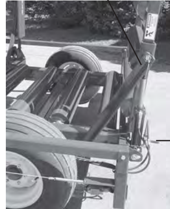
Tail/Ramp Hydraulic Locking Valve
