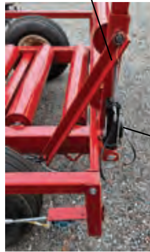
Tail/Ramp Hydraulic Locking Valve
