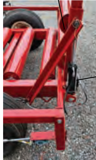
Tail/Ramp Hydraulic Locking Valve
