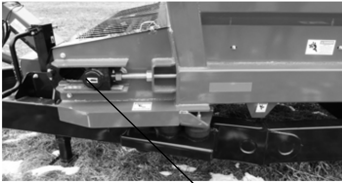
(1) Zerk on each end of front idler shaft
