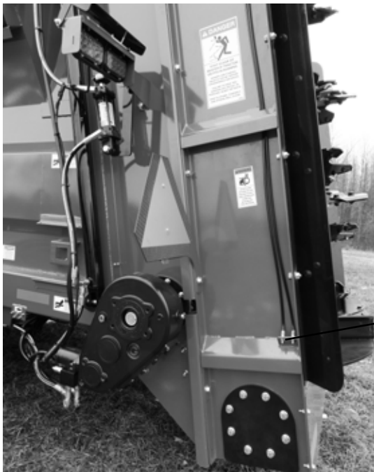
Remote Zerks (5) for the main drive shaft bearings under the spreader
