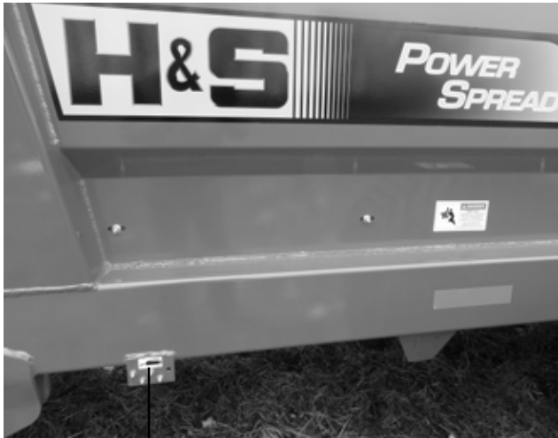
(1) Zerk on each end of front idler shaft
