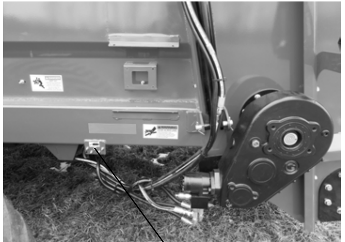
Remote Zerks Top LH Zerk - Left Side Tandem Pivot Bottom LH Zerk - Right Side Tandem Pivot Top Center Zerk - Rear Drive Shaft Bearing Bottom RH Zerk - Left Side Drive Shaft Bearing Top RH Zerk - Right Side Drive Shaft Bearing
