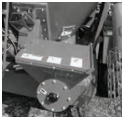
Supplement Hopper Auger Bearing (1 zerk)
