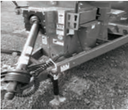
Telescoping PTO Drive (3 zerks)
