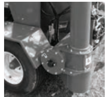
#1 Discharge Auger End Bearing (1 zerk)
