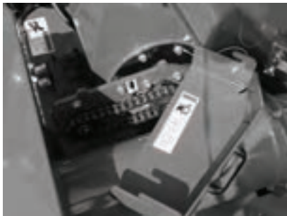
#1 Discharge Auger Bearing (1 zerk under shield)
