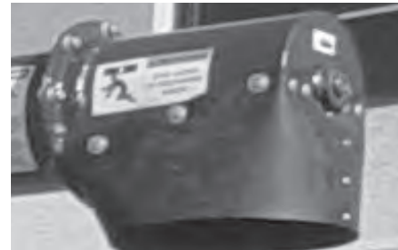
Unloading Auger- (1 zerk at the end of the auger discharge spout)
