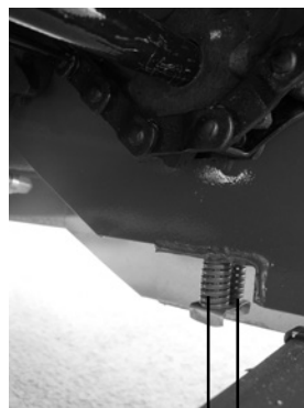
Rear Center Main Apron Tightener Bolts
