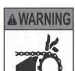
DO NOT OPERATE THIS EQUIPMENT IF THIS DECAL IS EXPOSED. REPLACE SAFETY SHIELDS.
