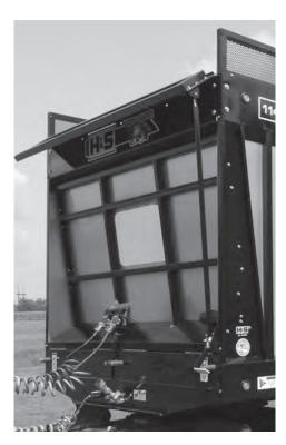
All **Top Dog** models have the capability of folding down the upper front panel for when harvesting ahead of the forage box.
