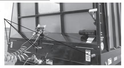
Tighten the full threaded bolts to adjust aprons. Aprons are properly adjusted when two cross slats, or about three feet of chain lift off the chain return slides from the front of the box. Maintain this when operating the box.
