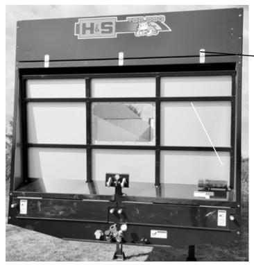
All **Top Dog** models have the capability of unbolting and folding down the upper front — panel for harvesting ahead of the forage box. An optional Electric Actuator for the fold down panel is available
