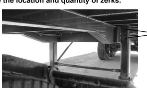
Landing Gear 2 zerks on the gearbox of each leg.
