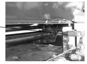
Tighten the full threaded bolts to adjust aprons. Aprons are properly adjusted when two cross slats, or about three feet of chain lift off the chain return slides from the front of the box. Maintain this when operating the box.
