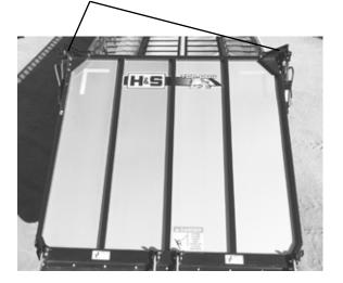
Doors 1 zerks on each hinge point of each door
