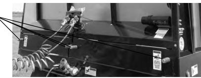
Tighten the full threaded bolts to adjust aprons. Aprons are properly adjusted when two cross slats, or about three feet of chain lift off the chain return slides from the front of the box. Maintain this when operating the box.
