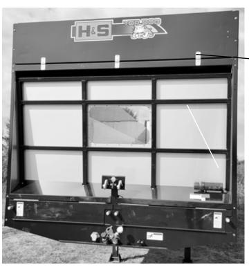
All *Top Dog* models have the capability of unbolting and folding down the upper front—panel for harvesting ahead of the forage box.
