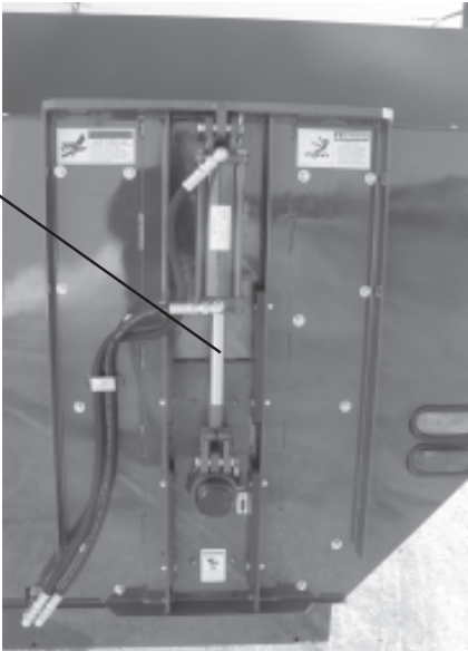
The discharge gate control cylinder shaft and both front and rear main auger cylinders should also be frequently coated with a rust preventative spray or lubricate since the cylinder shaft may remain extended when not being used for a period of time.
