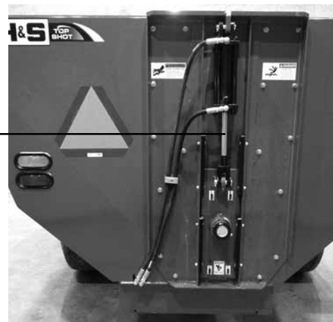
The discharge gate control cylinder shaft and both front and rear main auger cylinders should also be frequently coated with a rust preventative spray or lubricate since the cylinder shaft may remain extended when not being used for a period of time.
