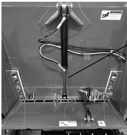
The discharge gate control cylinder shaft and both front and rear main auger cylinders should also be frequently coated with a rust preventative spray or lubricate since the cylinder shaft may remain extended when not being used for a period of time.
