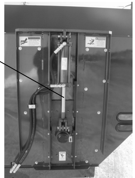
The discharge gate control cylinder shaft, discharge door deflector shield cylinder shaft and both front and rear main auger cylinders should also be frequently coated with a rust preventative spray or lubricant since the cylinder shaft may remain extended when not being used for a period of time.
