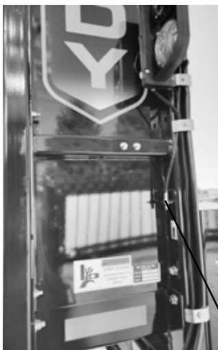
Top Pivot Door Remote Zerks (2) 1 zerk on each hinge point
