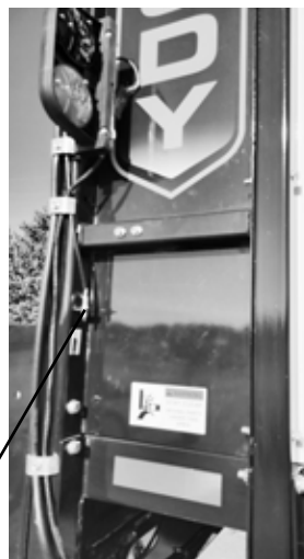
Top Pivot Door Remote Zerks (2) 1 zerk on each hinge point
